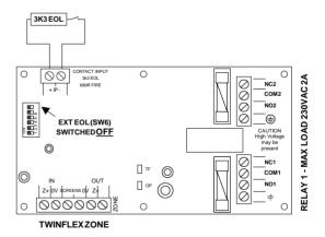
For use as a 'change-over' relay output with fault monitoring, connect to relay contacts and input as shown above, **remembering to set the External EOL switch to OFF**, and to use a volt free fault contact to break the EOL circuit in order to generate a fault condition.
