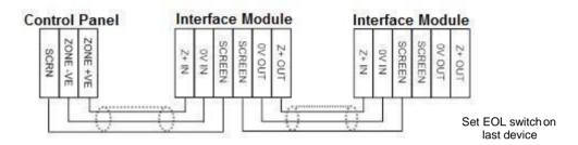
The MAGDUO Interface can be mixed on the same zone as other types of MAGDUO device. The above diagram shows how to make the zone positive, zone negative and screen connections between the control panel and the MAGDUO Interfaces. Refer to the instruction leaflets supplied with other MAGDUO devices for their equivalent wiring/terminal labelling details.
